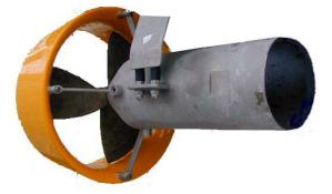
gland seal on the shaft. A transparent chamber controls the tightness. A second gasket protects the electric motor from a default of the rotating seal.
